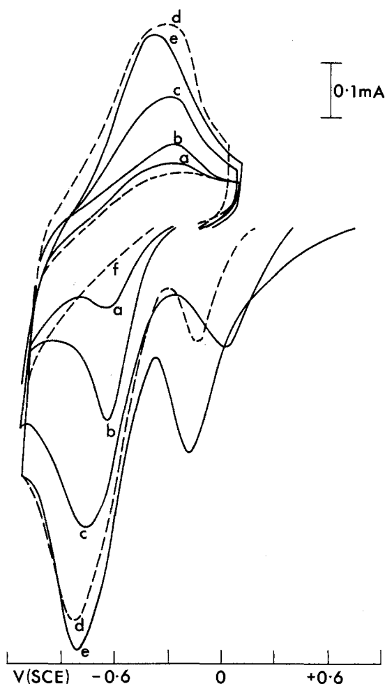
Fig. 1. Voltammograms obtained in a borate-boric acid buffer solution for stainless steel, Type 316L, anodized 1h in the buffer solution; specimen areas in \text{cm}^2 and anodizing potential in volts, respectively, are as follows: a: 3.4, 0. b: 3.8, 0.3. c: 3.9, 0.6. d: 4, 0.75. e: 3.8, 0.9. f: Specimen 3.8 \text{ cm}^2 in area exposed to air for 4h following initial cathodic reduction step.
