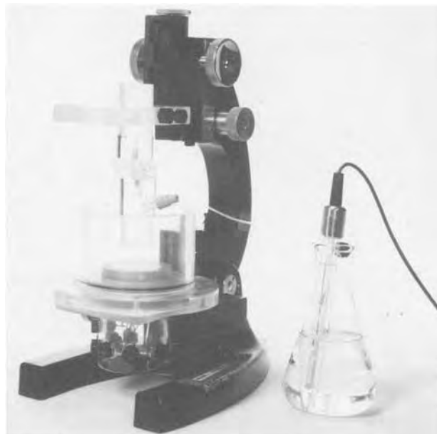
Fig. 2. Experimental crevice corrosion cell described in detail in Ref. (2).
