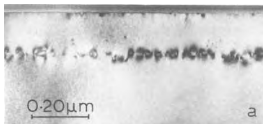
Fig. 17. Cross-sectional TEM micrograph of As ( 100 \text{ keV} , 1 \times 10^{16} \text{ cm}^{-2} )-implanted silicon after rapid thermal annealing at 1050^\circ\text{C}/10\text{s} .
