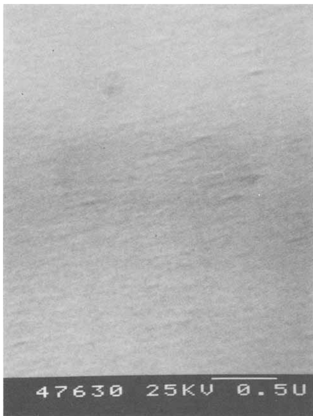
Fig. 3. Scanning electron micrograph of a thin film (2000Å) of poly(methylphenyl)silane cast on a silicon substrate.
