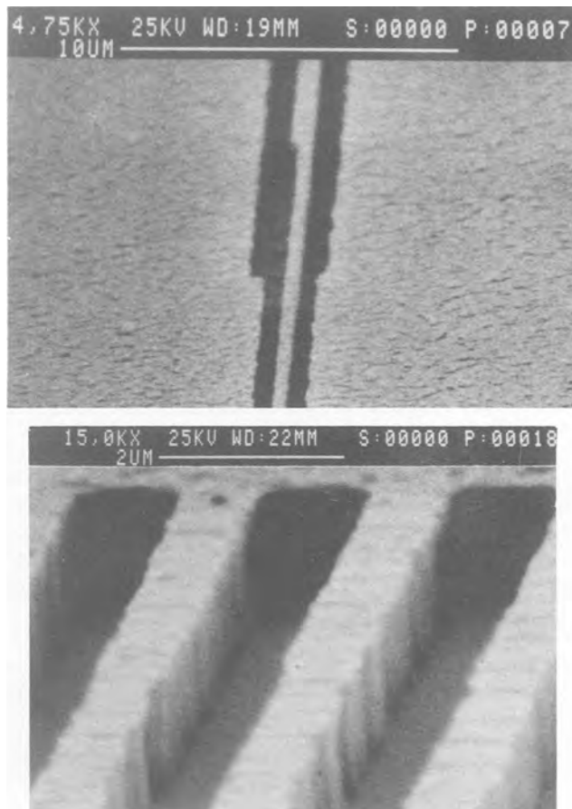
Fig. 2. Submicron pattern O 2 RIE'd into 1.2 \mu\text{m} -thick HPR-204 using terpoly(ATMS butene sulfone) as a top imaging layer
