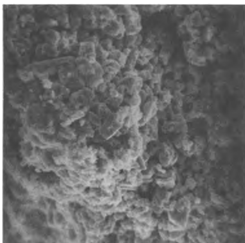
Fig. 12. Morphology of the interior of the electrode. Discharge with -30 \text{ A/m}^2 to -350 \text{ Ah/m}^2 .
