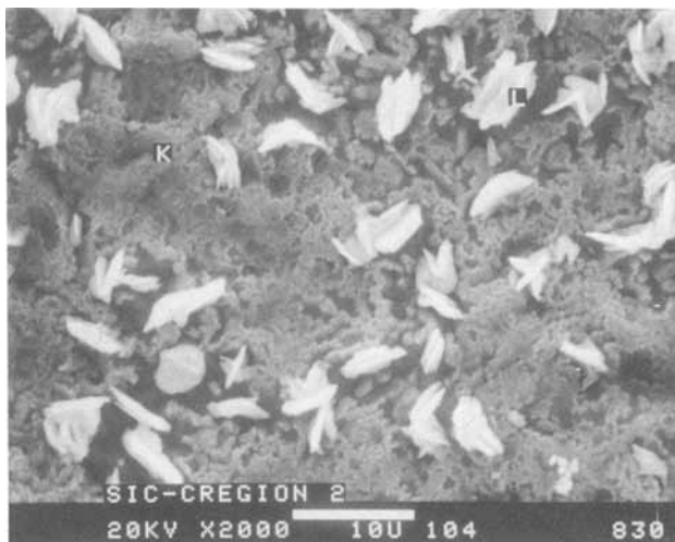
Fig. 9. Surface of SiC coating below \text{Na}_2\text{S}_5 melt level of sample SiC-C after 84 days at cathodic potential of 300 mV. Region K is amorphous SiC with "worn" look; areas L are platelike chromium sulfide crystals.
