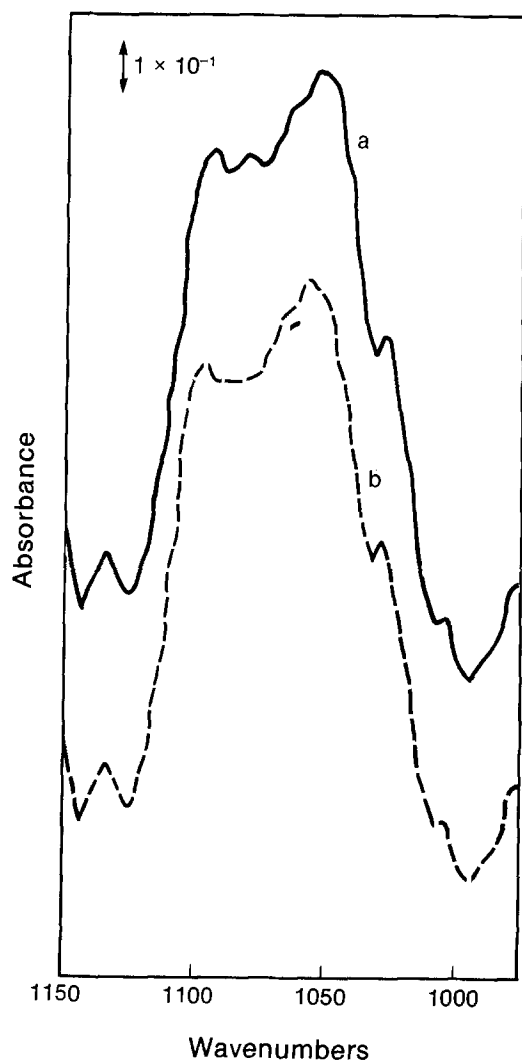
Fig. 4. In situ IR spectra of Pt surface in 1 \text{ mol dm}^{-3} \text{ HClO}_4 \text{ (aq.)} + 6.6 \times 10^{-3} \text{ mol dm}^{-3} \text{ H}_3\text{PO}_4 \text{ (aq.)} at (b) 0.0V and (a) 800 mV, before the subtraction of the solution spectrum.
