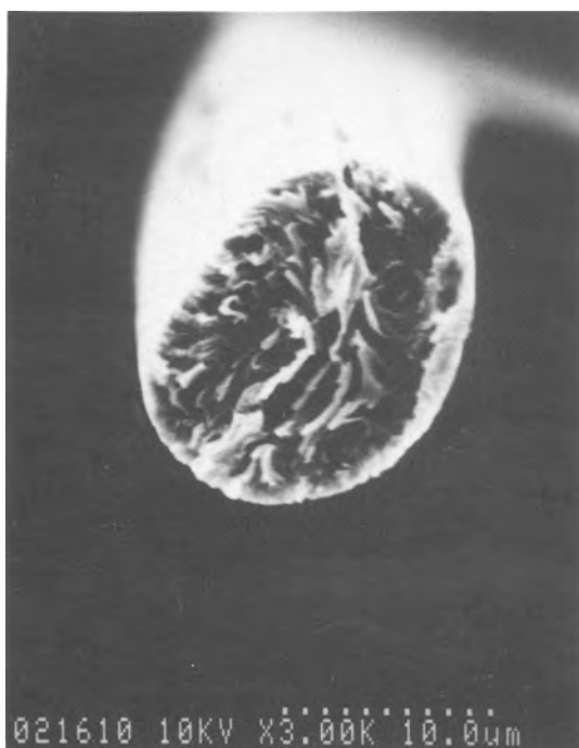
Fig. 1. SEM micrograph of cross section of the 3000°C treated mesophase-pitch-based carbon fiber.
