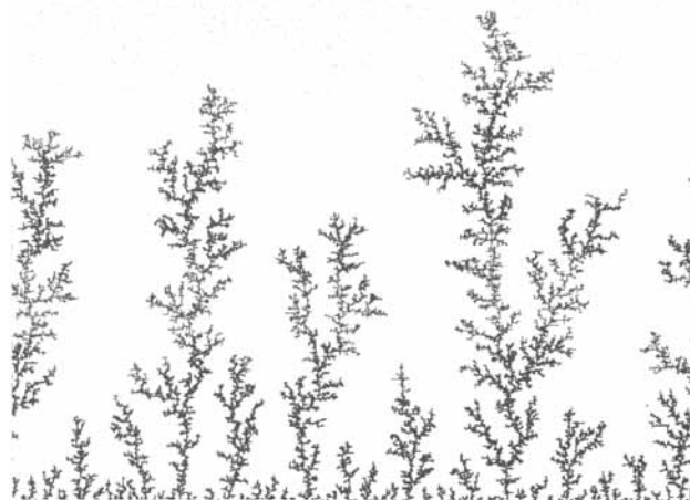
Fig. 1. Simulation of growth for concentration of 0.1 (fraction of occupied sites) and sticking coefficient of 0.3. The transition between black and gray indicates time evolution in units of 2 \times 10^5 Brownian motion steps.
