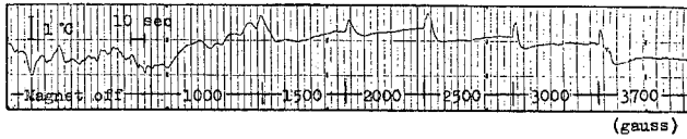
Fig. 3. Effect of magnetic field on temperature fluctuations in silicon melt, measured at 10 mm below the melt surface of the crucible center.
