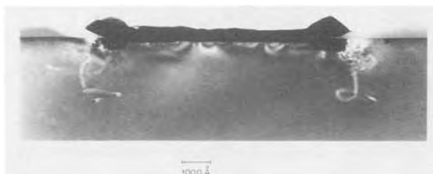
Fig. 13. TEM of a W film deposited on a window to Si on a tester device (wet-etched window). Note tunnels in the Si emanating from the window edges.
