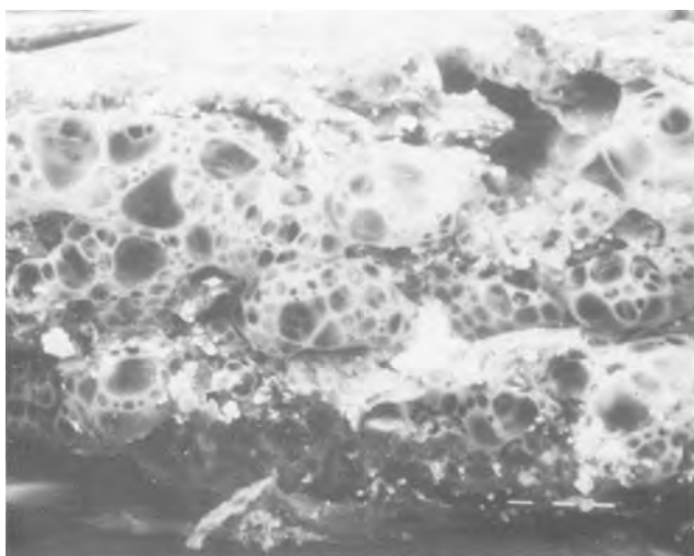
Fig. 9. Cross section of separator from cell 1 (Cd side at top, Ni side at bottom).
