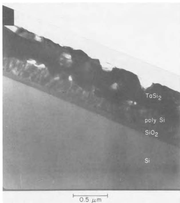
Fig. 21. TEM vertical cross section illustrating presence of voids at various levels of \text{TaSi}_2 film.
