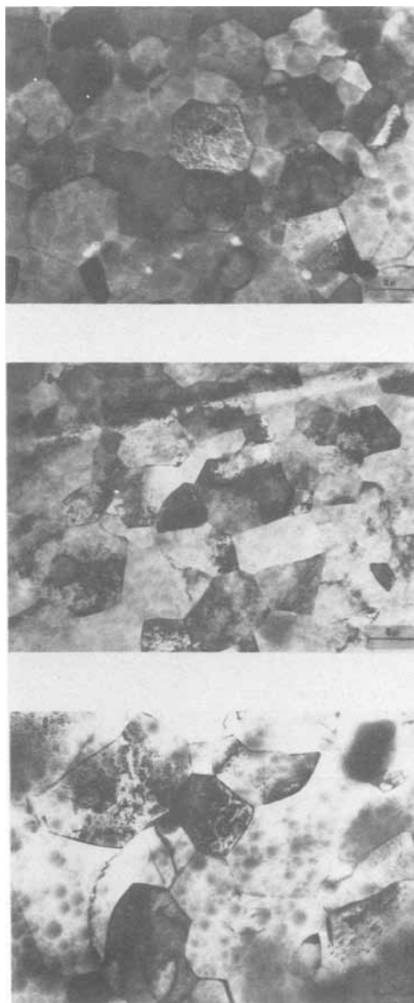
Fig. 11. TEM horizontal cross-sectional micrographs illustrating grain size and grain size distribution of In-Source Al-0.5%Cu deposited at 300°C at a rate of \sim 140 \text{ \AA/s} and sintered at (A) 300°C/30 min/ \text{H}_2 , (B) 300°C/30 min/ \text{H}_2 with additional 1.4 \mu\text{m} plasma SiN cap, and (C) 450°C/30 min/ \text{H}_2 .
