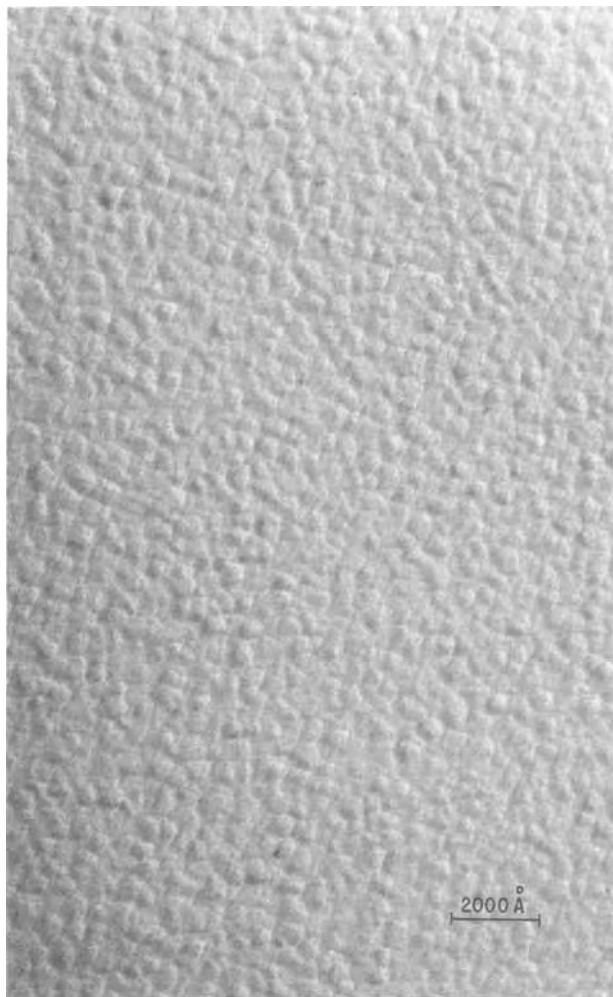
Fig. 1. Typical morphology of the organic solvent-based, Co-Fe-Cr-oxide spinel film at high magnification, showing the low profile structure. The electron micrograph is of a standard replica taken with a JEM-7 microscope.
