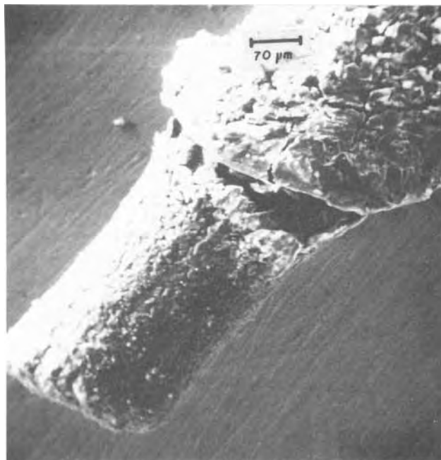
Fig. 5. SEM photograph of an iron tip removed from the solution a few minutes after mechanical oscillations started. The dark region (iron or iron oxide) surrounded by the lighter overlayer of iron sulfate was located just on the triple-phase boundary for the meniscus upper level.
